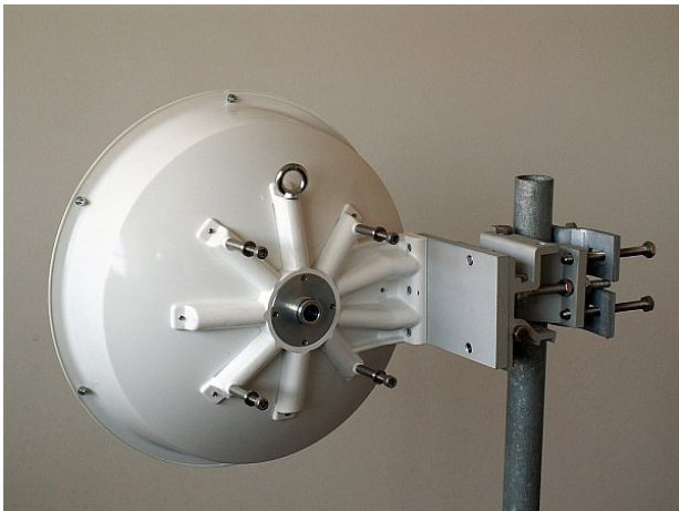
Fig. 5.14: Dish before installing the FOD unit
